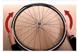
Pinch the rim's bead together and place it into gutter. Continue this around the wheel – pinch the tyres bead and force it into the rim's gutter, pulling the tyre away from the valve and towards the last bit of tyre you need to fit. This step is 90% of the magic.
