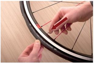
Now the tricks start: Start at valve and push the valve back into rim. We want the tyre's beads to be able to get into the rim's gutter so we're moving the valve out of the way as much as possible.
